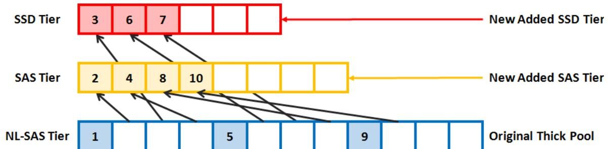
Figure 27 Block Map of Thin Provisioning Pool Transferring to Auto Tiering
